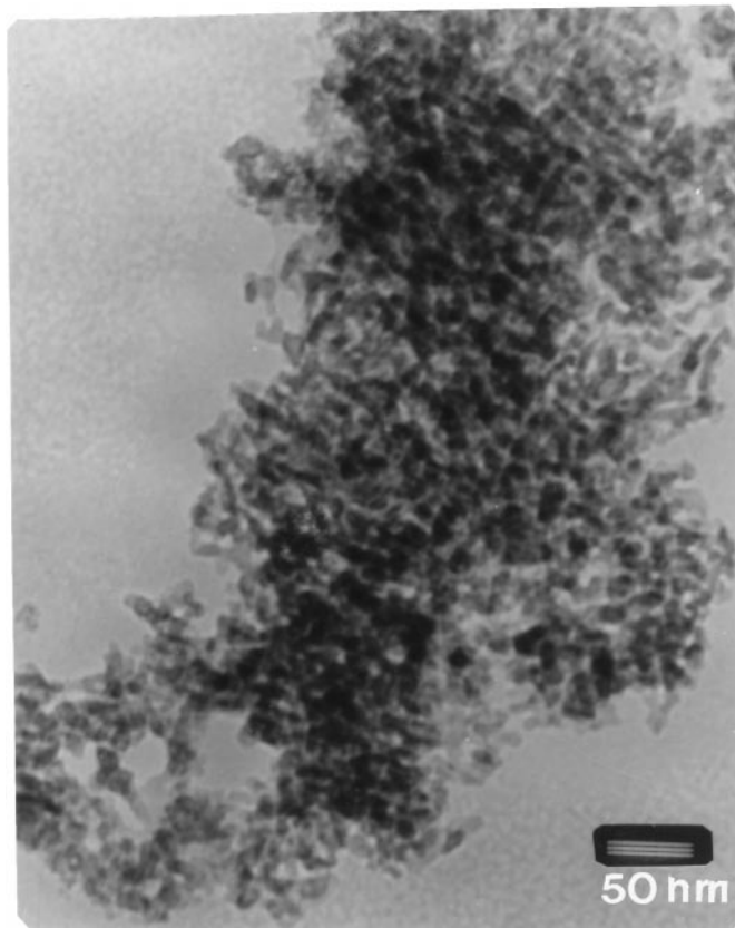
FIG. 9. TEM micrograph of the 1% Pt–18% TiO 2 –Al 2 O 3 catalyst.
