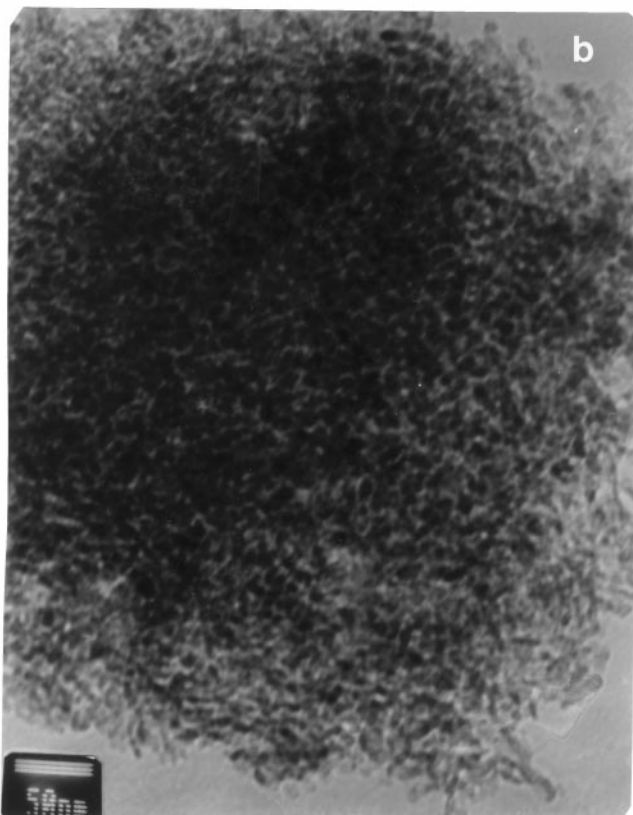
FIG. 7. The transmission micrographs of the 1% Pt-10% \text{TiO}_2\text{-Al}_2\text{O}_3 catalyst. Technique of (a) dark field and (b) light field.
